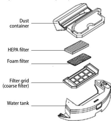
**Electrically operated water tank****Wiping module (clean after each use)**
